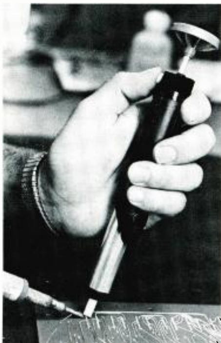
Fig. 5 Pneumatic device for removing solder.
