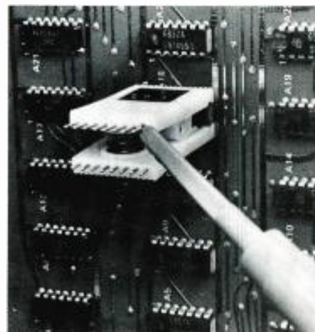
Fig. 4 Clamp-on "clothespin" for DIP's attached.
